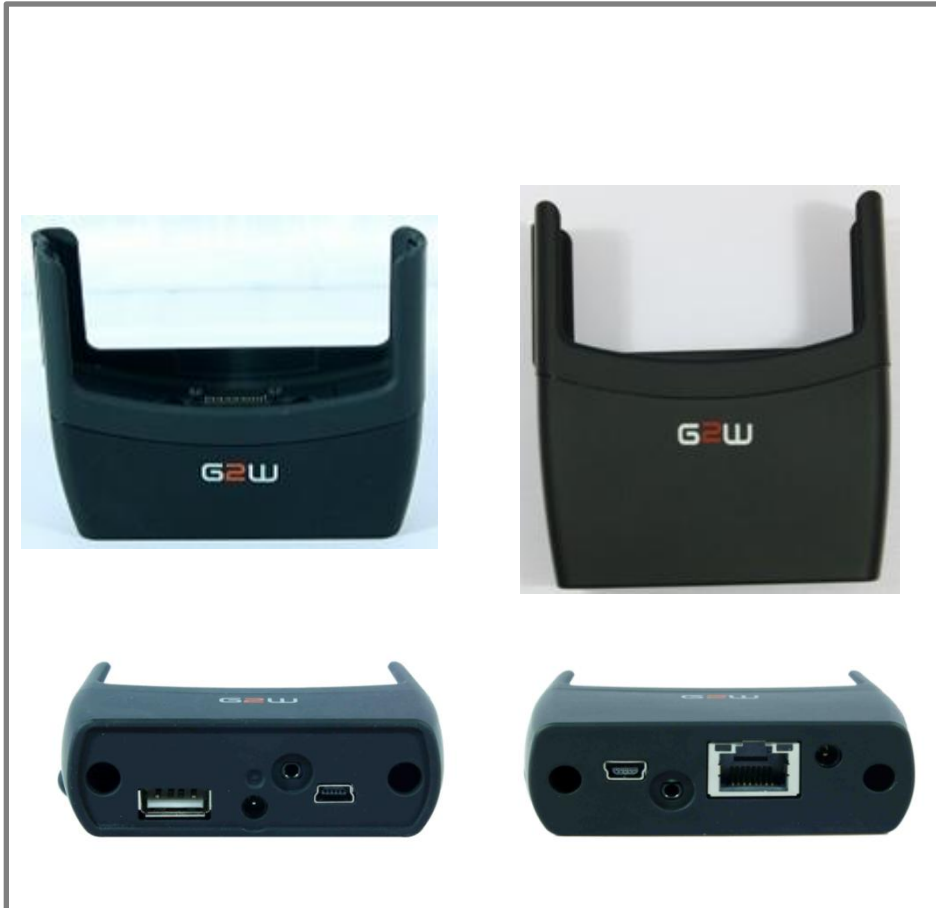
Snap-on Multi Gender with USB or with Ethernet DC Jack / Ethernet connector / Ear-phone Jack
